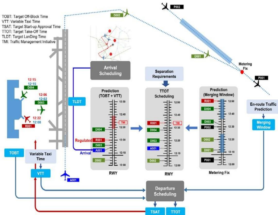
Figure2. Operational Concept of MIDAS
